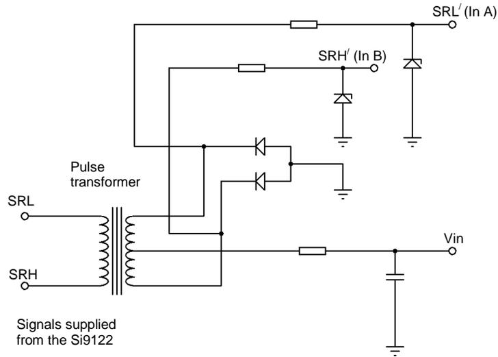
**Figure 6. Schematic showing powering intelligent driver from pulse transformer.**
