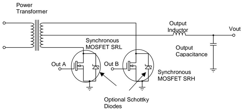
**Figure 8. Power stage of half-bridge converter**
