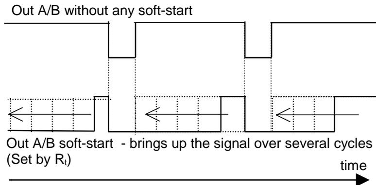
Figure 10. Soft-start of the output drivers.
