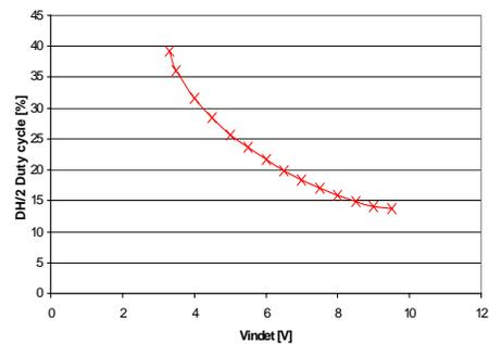
Figure 3. Example of the voltage feed forward control.
