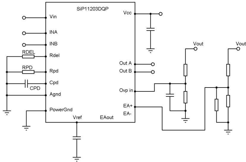
**Figure 12. Schematic showing application circuit of intelligent driver.**
